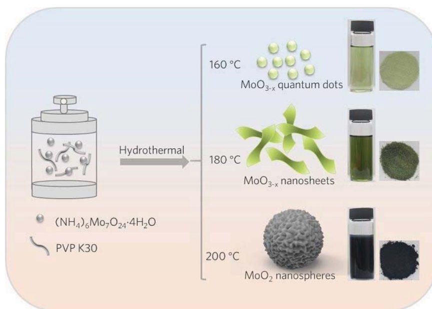
Figure 1. Schematic illustration describing the hydrothermal treatment synthesis process.
